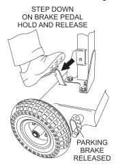
Figure 22. Parking Brake (Release Position)
